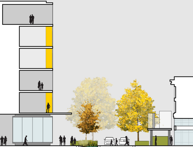
rain garden permeable pavement new frontage right of way
