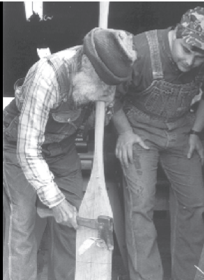
OZARK PADDLEMAKER ERNEST “UNCLE PUNK” MURRAY SHOWS APPRENTICE STEVE COOKSON HOW TO SHAPE A SASSAFRAS JOHNBOAT PADDLE, DONIPHAN, 1995. (PHOTO BY DANA EVERTS-BOEHM)
